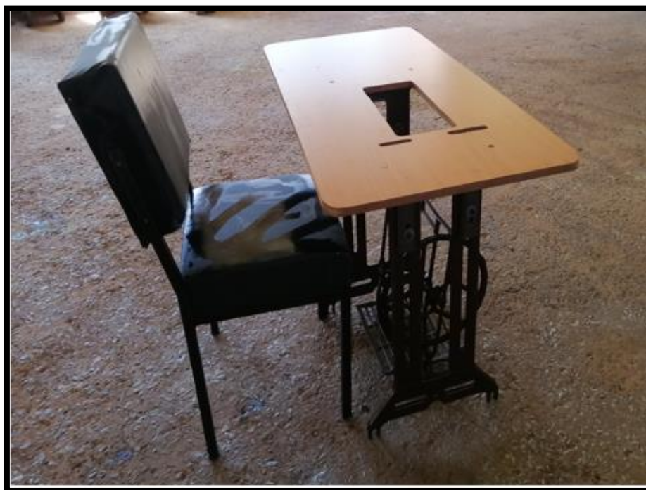
Figure 4.23: The complete assembling of the sewing workstation redesign
