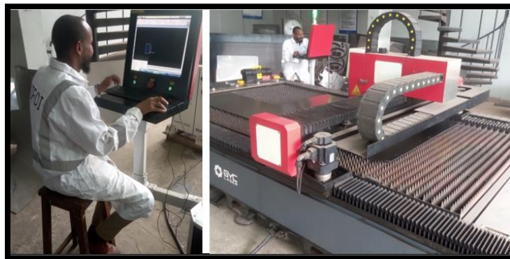
Figure 3.39: Cutting process using a laser cutting machine
