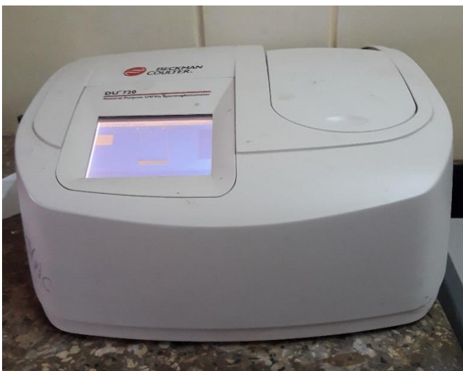
Figure 3.5: UV/Vis spectrophotometer ready for measuring dye absorbance
