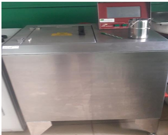
Figure 3.7: Gyrowash Machine for Carrying out Colourfastness to Washing
