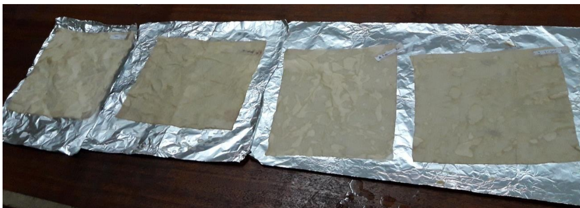
Figure 5. 2: Pre-Treated Cotton Fabrics with Keratin Hydrolysate
