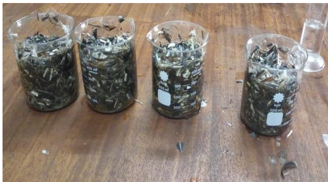
Figure 3.3 Dissolving of Chicken Feathers in Sodium Hydroxide Solution
