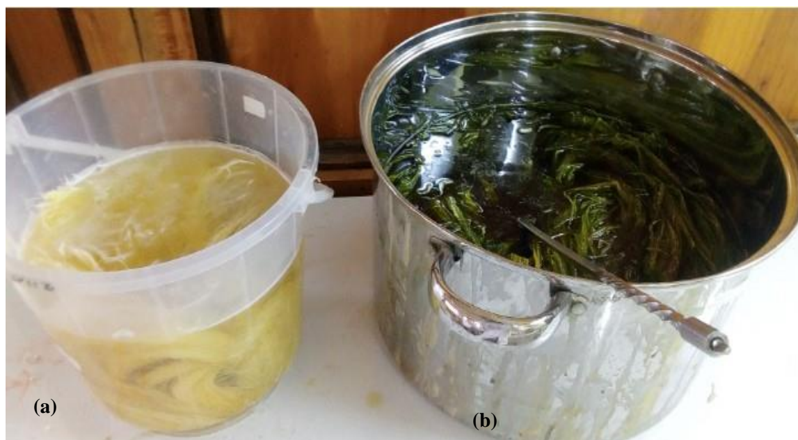
Figure 3.4: Alkali treatment of (a) Sisal and (b) Cattail fibres
