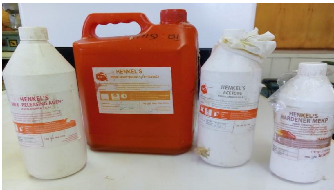
Figure 3.3: Precursor for synthesis of sisal/cattail hybrid composites: Mould release agent, Polyester resin, Acetone and Hardener (MEKP)
