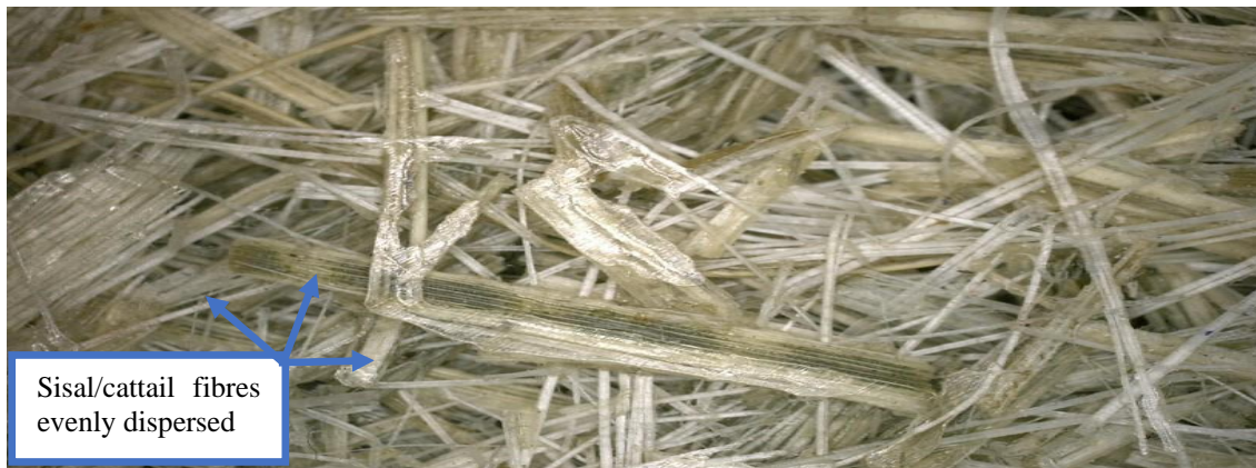
Figure 4.4: Micrograph of hybrid composite with 15wt.% and constant percentage of sisal/cattail fibres in the composite.
