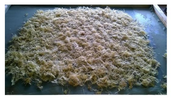
Figure 14: The random dry-laid web from *luffa cylindrica* fibres
