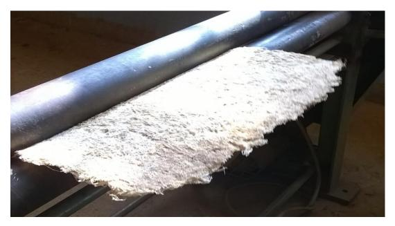
Figure 16: Consolidating the nonwoven structure from *luffa cylindrica* fibres
