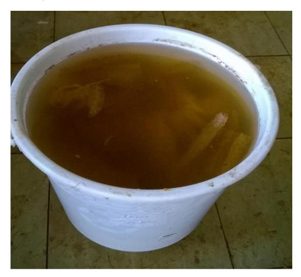
Figure 13: Water retting of *luffa cylindrica* fibres
