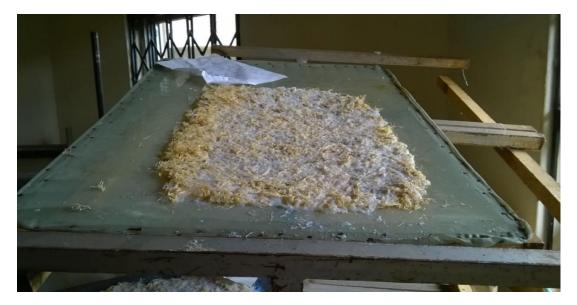
Figure 15: The adhesively bonded web from *luffa cylindrica* fibres
