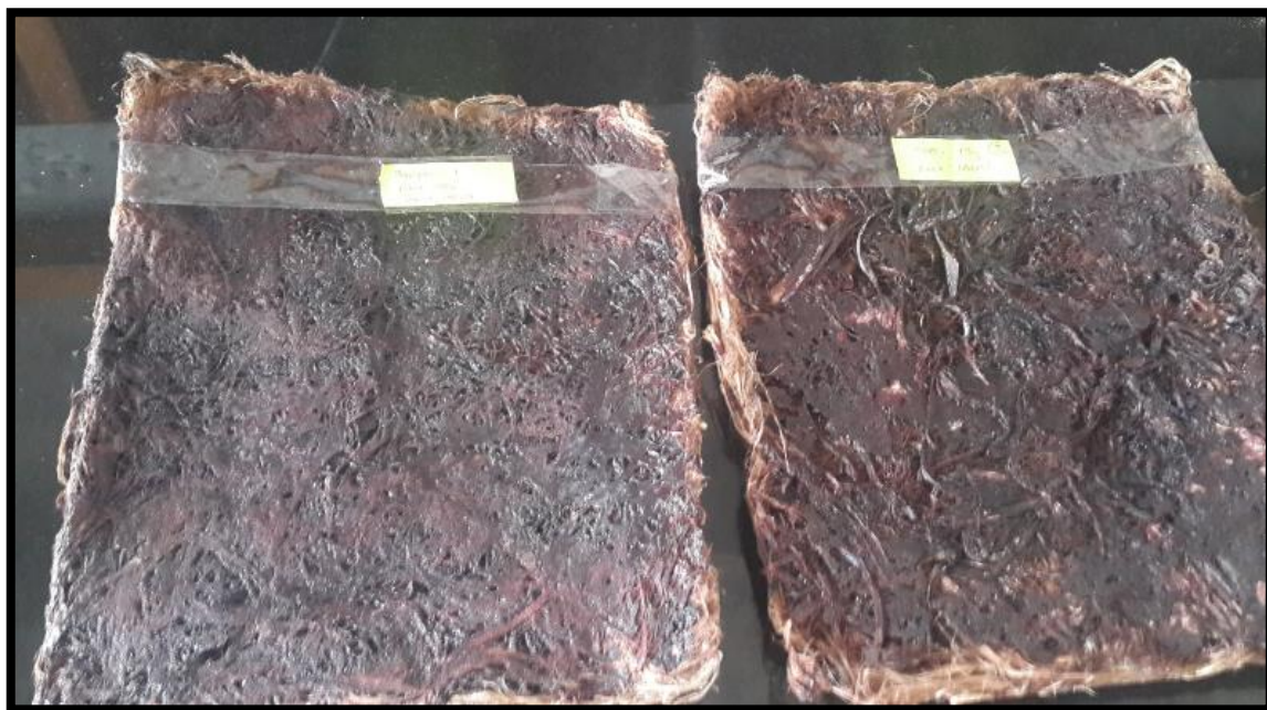
Figure 4-14 – Samples of fabricated fibreboards
