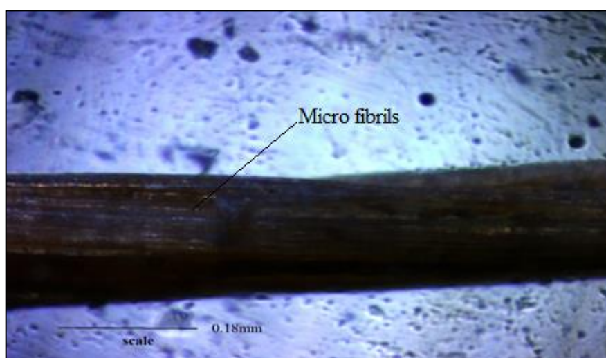
Figure 4-6 – Cross sectional microscopic image of cotton stalk fibre x10 magnification Image J software was used to scale the fibre and take measurements of its mean diameter. The mean fibre diameter of these fibres was 0.189 mm. Table 4-3 shows the fibre diameter measurement that was taken for top section cotton stalk fibre. The mean fibre diameter of these fibres was 0.189 mm.
